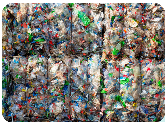
Figure 19. From top to bottom: a stack of sorted bales of HDPE and PP, and in detail.
