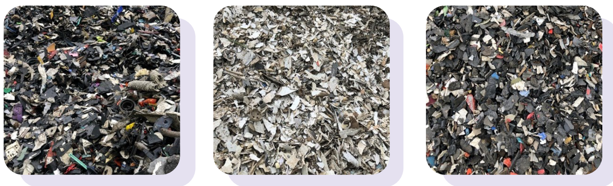
Figure 15. Top to bottom: ASR from ELV, SLF from mixed WEEE and SLF from temperature exchange equipment. These are the fractions entering the recycling line (see Recycling technologies chapter).
