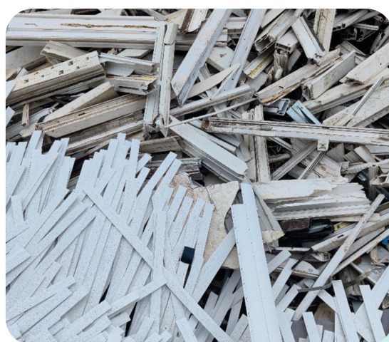
Figure 43. Mixed windows and door profiles, a typical incoming PVC rigid waste.
