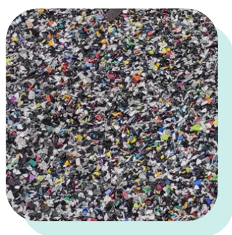
Figure 41. Output WEEE fraction of the first sink/float bath, i.e., the one separated from the 'heavy fraction' (contaminated plastics).
